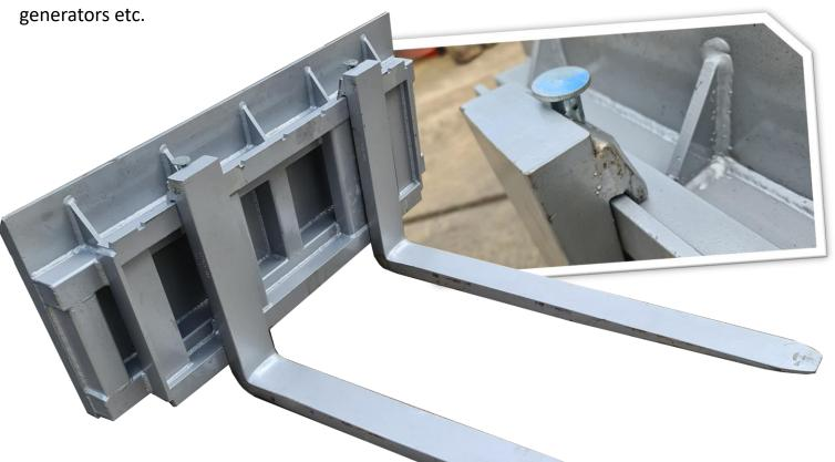
Universal Skid Steer Hitch Pallet Forks **Type** Width 975mm Depth 1.230mm 540mm Height **Fork Length** 1,070mm **Adjustment Width** 120-790mm **Machine Weight** 120kg Up to 800kg **Load Capacity**
